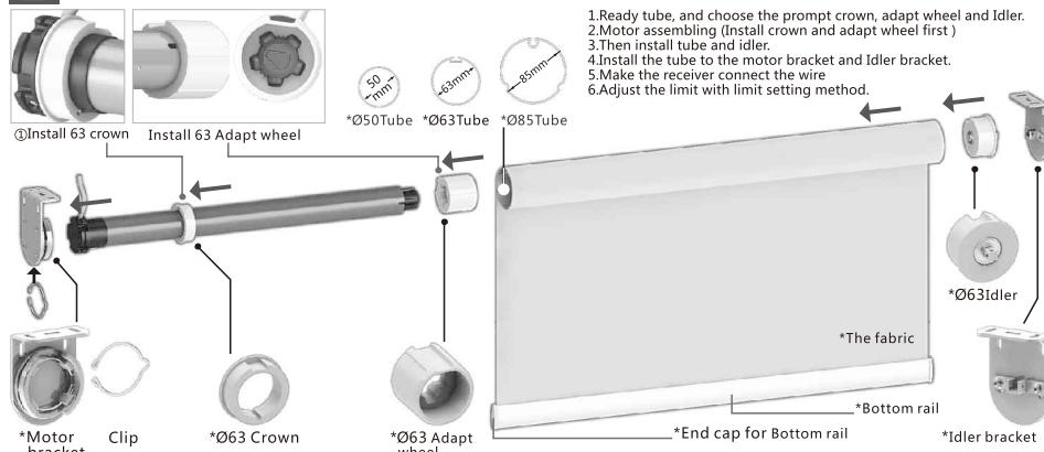
Note: Try to operate the whole roller blinds after installation, especially to check the fabric straight or not.
