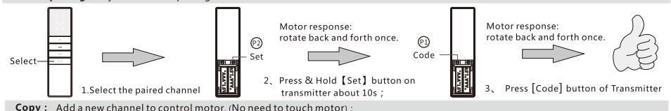
**Copy :** Add a new channel to control motor. (No need to touch motor) :
