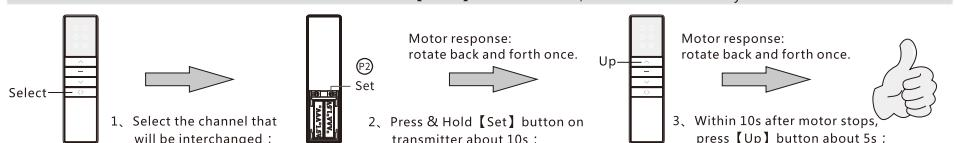
**L limit travel adjustment method** \*First adjust Down-limit travel and then up-limit travel.
